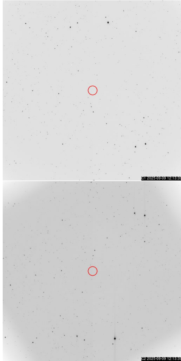
Figure 3.1: Typical images in the blue channel (above) and red channel (below). Note that the red channel is flipped vertically with respect to the blue channel because of the reflection off the second dichroic. Note also the vignetting in the red channel caused by the incorrect orientation of the filters and the trails above and below bright stars.
