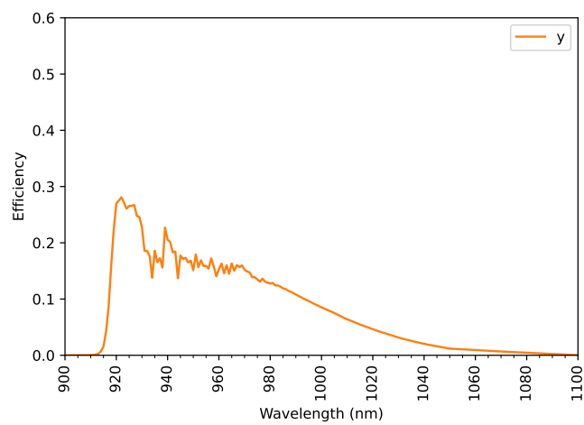
Figure 7.6: The system efficiencies in the z and y filters.
